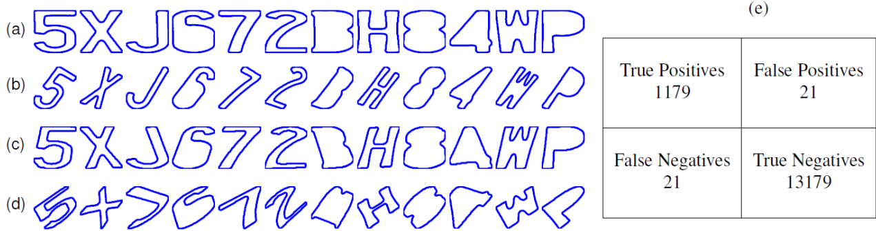
Figure 4: Contour images from the license plate database [1]. The digits extracted from license plates as seen at (a) Camera 1, (b) at a randomly generated viewpoint of the curves observed at Camera 1, (c) at Camera 2, and (d) at a randomly generated viewpoint of the curves observed at Camera 2. (e) Confusion matrix for 100 random projective transformations of curves in the license plate database.
