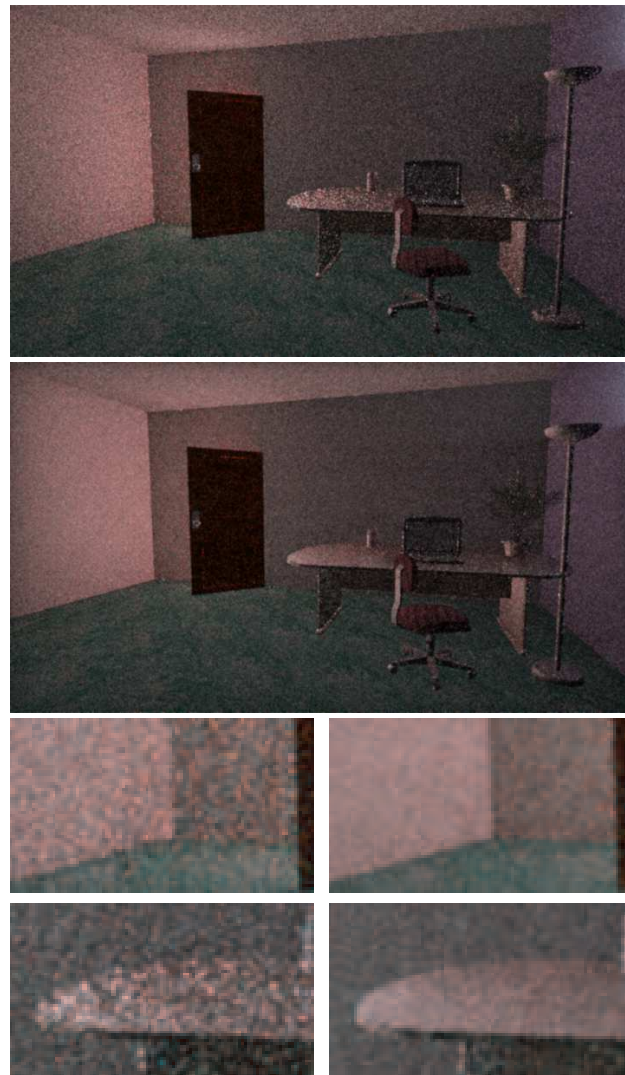
Figure 4.3: An example of variance control due to the user path proposal strategy. Top is the image rendered with no user paths, while center is the result when the user specified ten paths passing through the doorway. Bottom are zooms of the wall intersection and table regions, with no user paths on the left and user paths on the right. These are MLT images that directly visualize the sampled light paths. The improvements after a final gather, while present, are less apparent.
