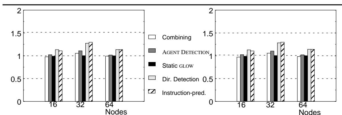
Figure 4.38. Normalized speedup (over SCI) for BARNES for 2 and 3 dimensions (16 to 128 nodes).
