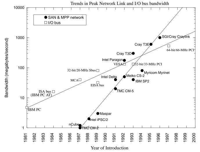
This figure shows the crossover point between peak System Area Network (SAN) and MPP network link bandwidths and "standard" I/O bus bandwidth. SAN and MPP link bandwidths have been increasing by roughly 100% per year, while the I/O bus bandwidth has been increasing by roughly 32% per year.
