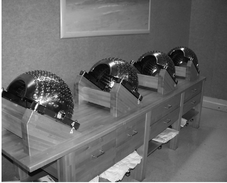
FIGURE 4. Stored Focussing Helmets for 4mm, 8mm, 14mm and 18mm shots
